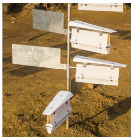
Dust catchers for monitoring and characterising air erosion in mine impacted soils
